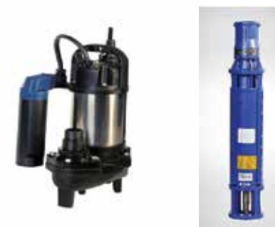
Portable submersible pumps with vortex impeller, wide pump casing for pumping sewage and waste containing fibrous material, solids and submerged debris.
