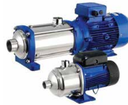
Non-self-priming, end-suction, multistage, high pressure centrifugal pump with axial threaded inlet and radial threaded outlet
