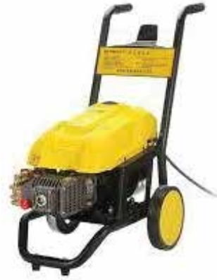
HBX W7/15 3Phase, Germany 5Hp, 380V, 1420Rpm, 3.2Kw, 10.5Amps, 12Lpm, 2100Psi
