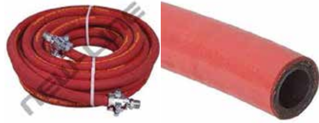
4inch, 100mm inner diameter, 200Psi, high tensile steel wire reinforcement.
