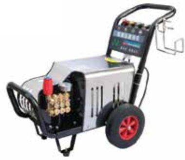
Pioneer/Hisaki Single phase, China 5Hp, 240V, 2800Rpm, 3.2Kw, 21Amps, 10.7Lpm, 2600Psi
